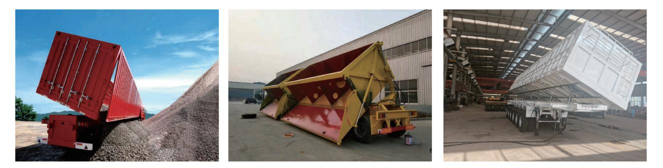
Side tipper trailer is a special type of dump semi-trailer that allows cargo to be unloaded laterally from one side of the semi-trailer. This type of semi-trailer is usually used to transport various goods that need to be easily unloaded, such as construction materials, agricultural products, lumber, etc.
