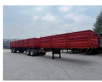
Unlike ordinary side dump trailers, the B Train Trailer---side tipper trailer is made up of two side dump trailers connected together, so it can accommodate a large amount of cargo. It can carry large amounts of bulk materials in one transport, making it ideal for large-scale bulk cargo transportation, especially where high efficiency and cost savings are required.
